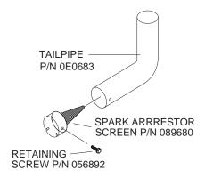
Figure 2.12 — Spark Arrestor Installation
